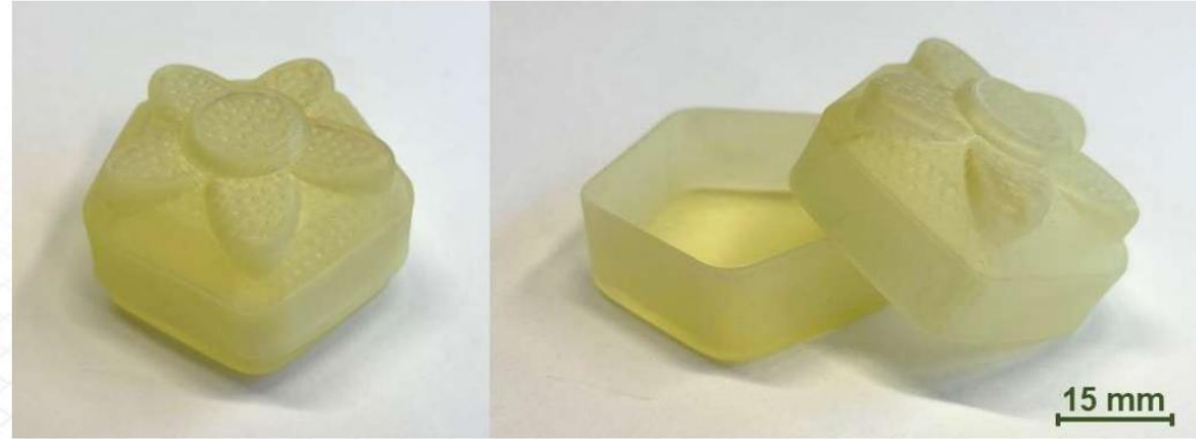
A box printed using an LCD 3D printer from a resin prepared on the basis of glycerol 1,3-diglycerolate diacrylate.
